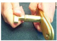
With the handle and escutcheon plate in their installed positions, make sure the set screw is on the bottom. Optional: While holding the handle tight to the extension, use a #29 or 1/8-inch drill bit in the set screw hole to carefully make a dimple in the "male" end of the handle. This will ensure that the set screw holds the handle securely in that exact location.
