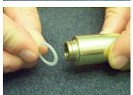
Place the washer from **Step 2** on the end of the extension piece. Or you can use a new washer from the kit.
