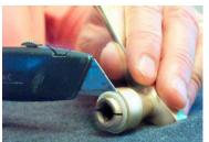
Use the blade of a box cutter to remove the nylon washer from the collar of the handle. Save the washer for later.
