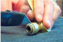
Using a thin blade (like a box cutter), remove the nylon washer from the collar of the handle. Save the washer.
