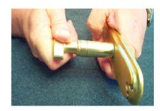
With the handle and escutcheon plate in their installed positions, make sure the set screw is on the bottom
