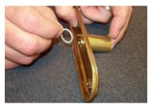
Insert the extension through the hole of the escutcheon plate. Now place another nylon washer on the extension.
