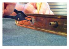
Remove the escutcheon plate from the door and save the screws. Using snap ring pliers, remove the snap ring and nylon washer from the back of the escutcheon plate.
