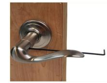
Replace the door handle. Line up the hole in the handle over the extension set screw. Turn the screw counterclockwise until the handle is secure.
