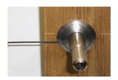
Slide on the extension. Line up the hole on the barrel of the extension with the set screw. If the set screw does not appear in the center of the hole, tap the end of the extension with a hammer until it does. Now turn the set screw clockwise until the extension is secure.
