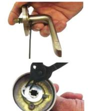
Remove the handle from the door. Loosen the set screws while holding the spindle in place.
